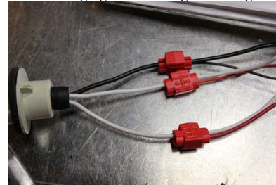
3-wire Parking light & Turn signal Wiring
